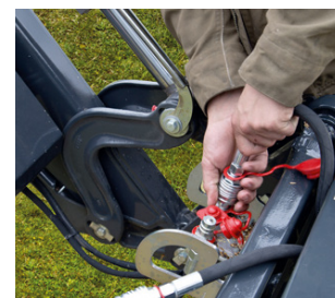
3 Plugging in the hydraulic connection.
